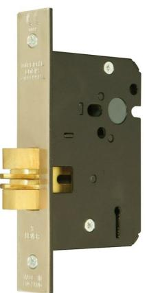
**Description** 3 Lever standard case mortice sliding door lock for use on internal wooden sliding doors providing a standard level of security. CE Marked door lock Fire rated to BS EN 1634-1:2000 & Performance rated to BS EN 12209. Bolt operated by key from either side. Supplied with 2 keys, striker plate and fixing screws. Finishes stainless steel (SS) or satin brass (SB). Other finishes available. 100 standard differs.
