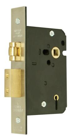
**Description** 5 Lever bushed keyhole mortice roller bolt sashlock for use on external wooden hinged doors providing a high level of security. CE Marked door lock Fire rated to BS EN 1634-1:2000 & Performance rated to BS EN 12209. Roller bolt operated by lever handle from either side Deadbolt operated by key from either side. Supplied with 2 keys, striker plate and fixing screws. Finishes stainless steel (SS) or satin brass (SB). Other finishes available. 1000 standard differs.
