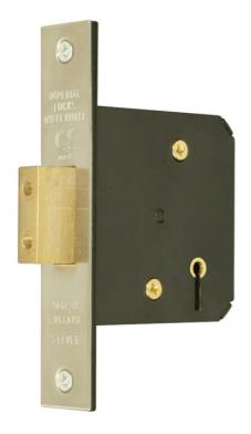
**Description** 5 Lever bushed keyhole mortice deadlock for use on external wooden hinged doors providing a high level of security. CE Marked door lock Fire rated to BS EN 1634-1:2000 & Performance rated to BS EN 12209. Deadbolt operated by key from either side. Supplied with 2 keys, striker plate and fixing screws. Finishes stainless steel (SS) or satin brass (SB). Other finishes available. 1000 standard differs.
