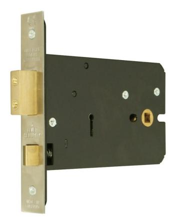
**Description** 5 Lever horizontal mortice lock for use on external wooden hinged doors providing a high level of security. CE Marked door lock Fire rated to BS EN 1634-1:2000 & Performance rated to BS EN 12209. Latchbolt operated by knob from either side Deadbolt operated by key from either side. Supplied with 2 keys, striker plate and fixing screws. Finishes stainless steel (SS) or satin brass (SB). Other finishes available. 200 standard differs.
