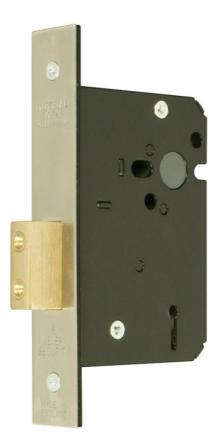
**Description** 5 Lever standard case mortice deadlock for use on external wooden hinged doors providing a high level of security. CE Marked door lock Fire rated to BS EN 1634-1:2000 & Performance rated to BS EN 12209. Deadbolt operated by key from either side. Supplied with 2 keys, striker plate and fixing screws. Finishes stainless steel (SS) or satin brass (SB). Other finishes available. 200 standard differs.
