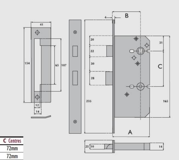
OPERATION: Latchbolt operated by lever handle from either side.
